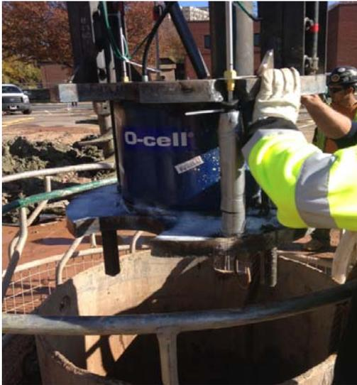
Fugro Loadtest was employed to provide foundation testing experience and equipment to Seaboard Foundations, Inc. in order to optimize the design parameters for foundations of the new building. Full scale O-cell load testing was performed prior to the ground breaking ceremony on a 29 m deep bored pile. Construction of the pile included multiple casings in the overburden soils and a 2 m long socket into bedrock.
