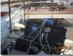
Automated O-cell Test Apparatus
