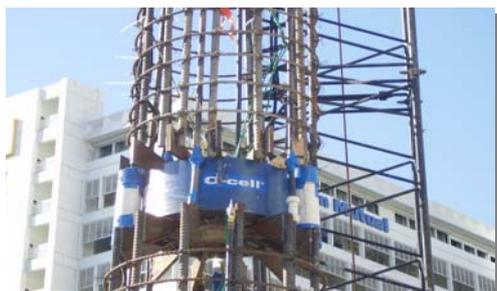
CFA test pile O-cell assembly ready for placement
